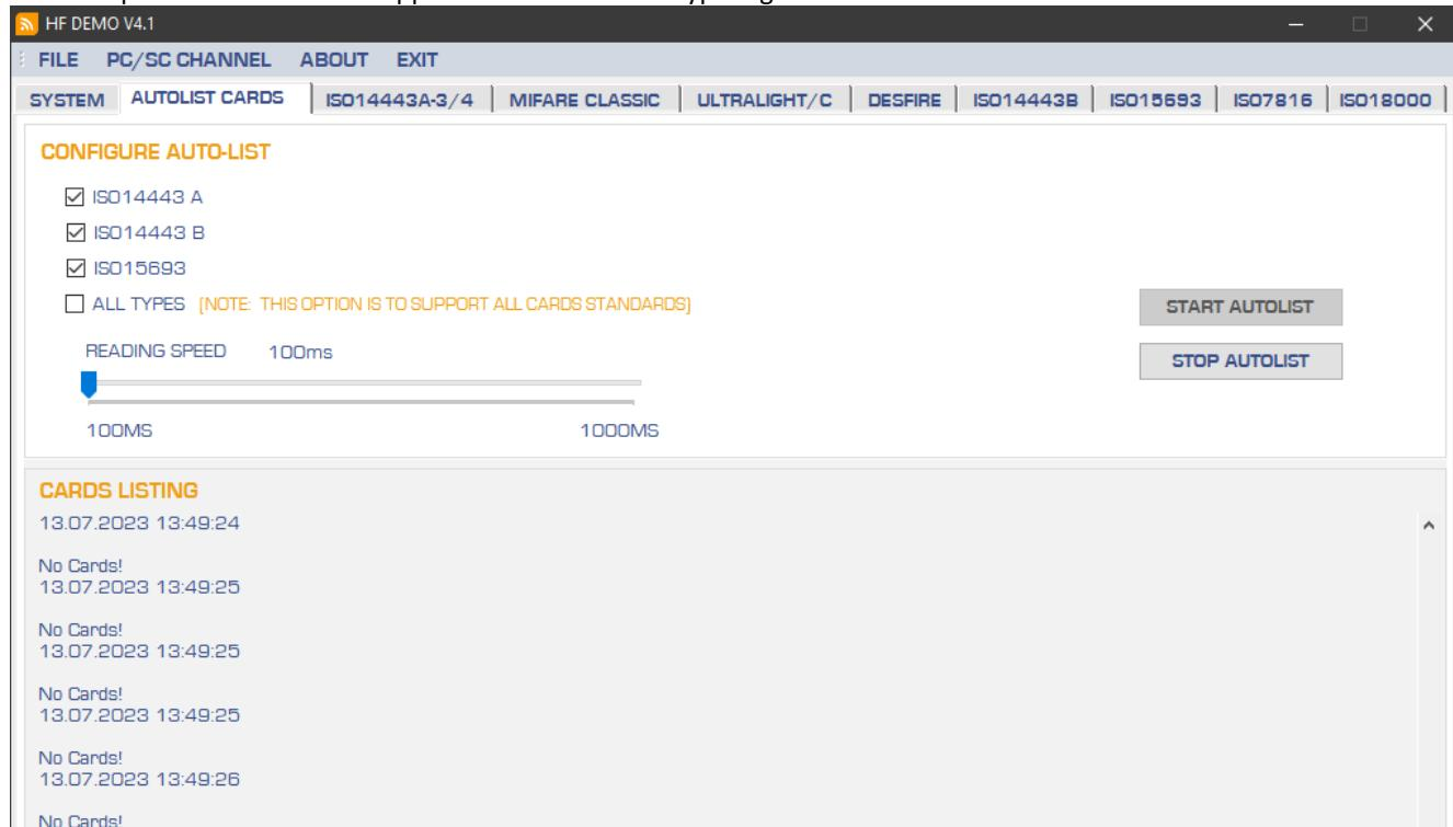
Please enlarge the reading speed to more than 150 ms for successful detection of ISO 15693 type tags:
